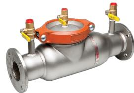
Series 2000SS Double Check Valve Assemblies are designed to prevent the reverse flow of polluted water from entering into the potable water system. This series can be applied, where approved by the local authority having jurisdiction, on non-health hazard installations. Features short end-to-end dimensions, lightweight stainless steel body, and low head loss.
