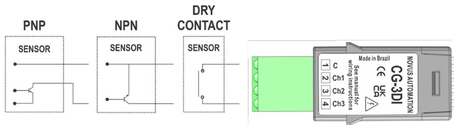
Figure 2 – Electrical connections
